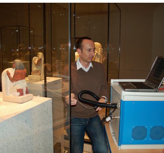
Figure 1 Real-time PTR-MS measurement in a gallery carried out by J. Kames. The capillary is entering the showcase via an interstice at the doors gasket
